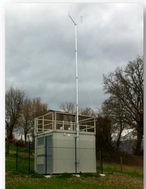
PTAP10-80 Meteorological pole h=10m compliant to WMO for environmental monitoring applications
