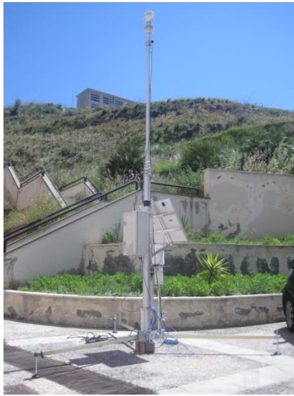
PTAP6-80 – Pneumatic telescopic pole h=6m with tripod and sonic anemometer with on-board compass
