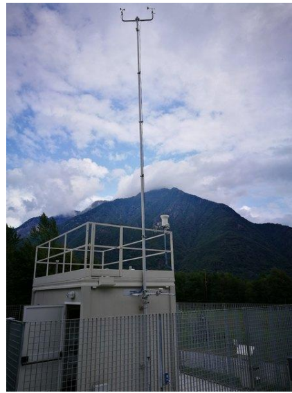
PTAP10-80 – Pneumatic (aut. Or manual) telescopic pole h=10m for air quality monitoring shelter
