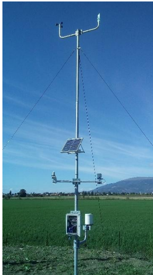
PF5-55 - Pole h=5m with guy wires
