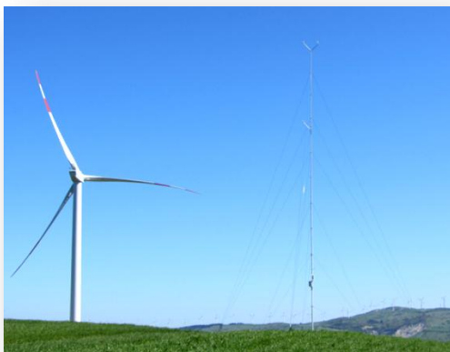
PRF20-60 Anemometric pole h=20m for wind turbines applications compliant to IEC61400-12
