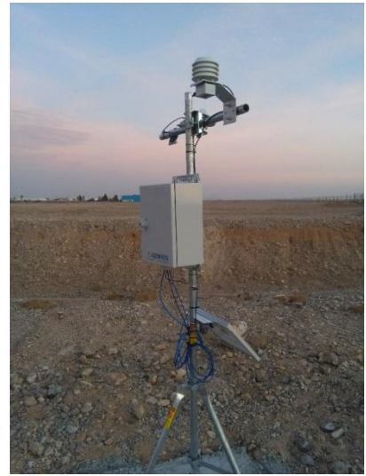
PL2-TREP – Light telescopic pole hmax=2.2m with tripod, fixing with ground stakes or concrete plugs
