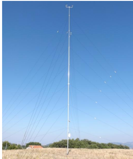
PRF15-60 – Anemometric pole h=15m with guy wires and without civil works
