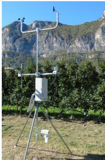
PL3-TREP – Light telescopic pole hmax=4m with tripod, screw tip base and ground stakes mounting
