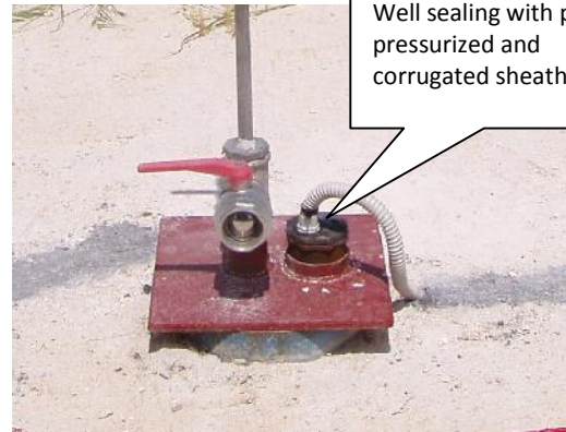
Example of installation in piezometric well for groundwater monitoring
