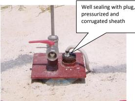
Example of installation in piezometric well for groundwater monitoring
