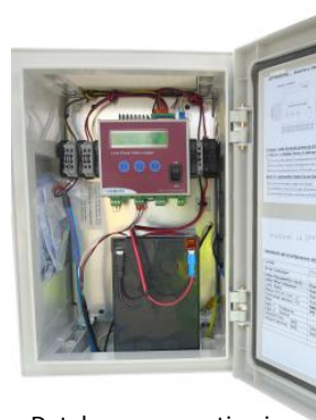
Datalogger mounting in the IP65 container
