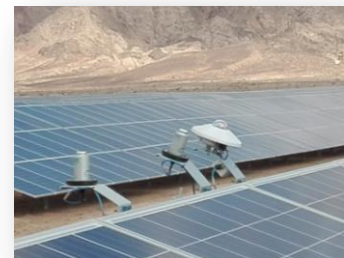
Particular of thermopile and silicon cell pyranometers – Jordan Installation
