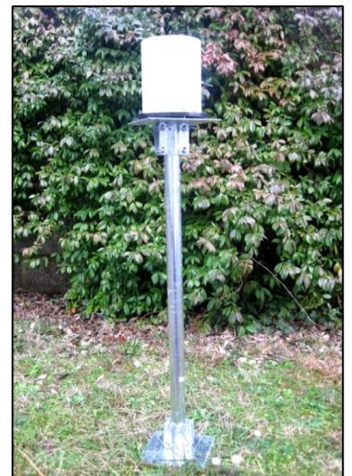
Rain gauge installation raised from the ground with support cod. SPL100 (h=100cm, ø45mm)
