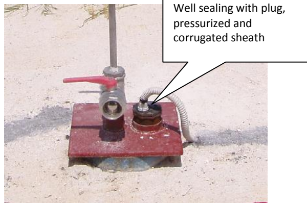
Example of installation in piezometric well for groundwater monitoring
