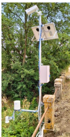
Examples of installation with 3m poles (with webcam, rain gauge and warning lamp)
