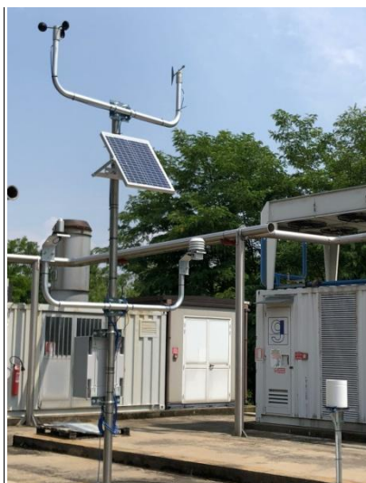
PF3-55 - Pole h=3m with base for fixing on the plinth or concrete pavement
