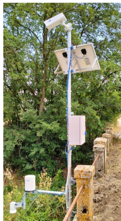
Webcam for hydrometric station with fastening on pole
